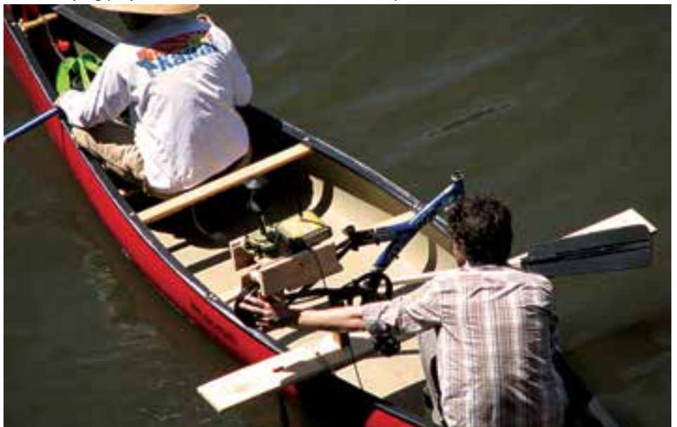
Our surveying project in 2010 included a home-built depth sounder.
